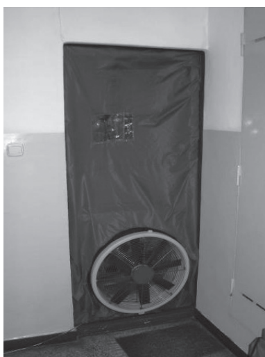
Ill. 1a. Blowerdoor set the in the Flat number 1
