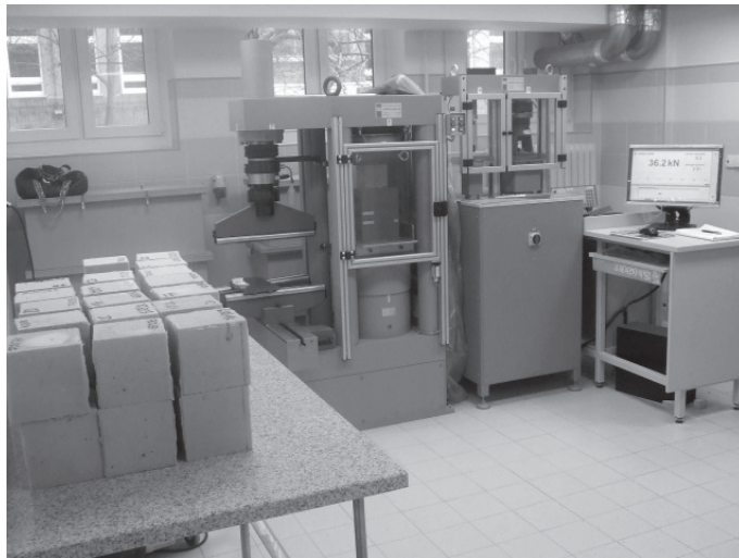
III. 3. Measurement of compressive strength
