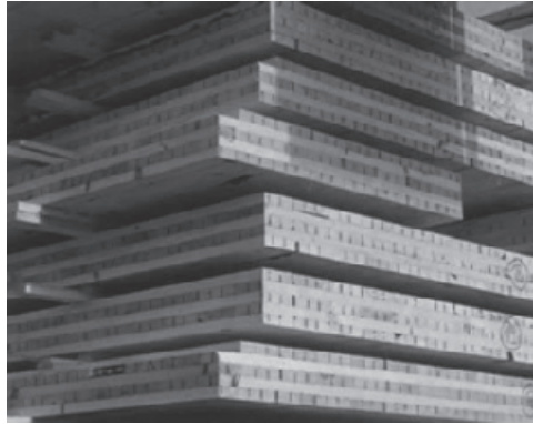
III. 12. Timber glued elements [13]
