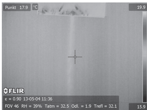
Ill. 6b. System joint – leak in place of vertical joint in building number 1
